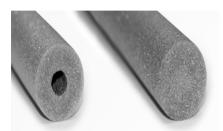
NOMATEC® Backer Rod Hollow & Full round profiles are manufactured from closed-cell polyethylene foam and are used as backing material for elastomeric and other cold-applied sealants. They are inserted into a joint to control the sealant depth and act as bond-breakers, without adhering to the sealant.
